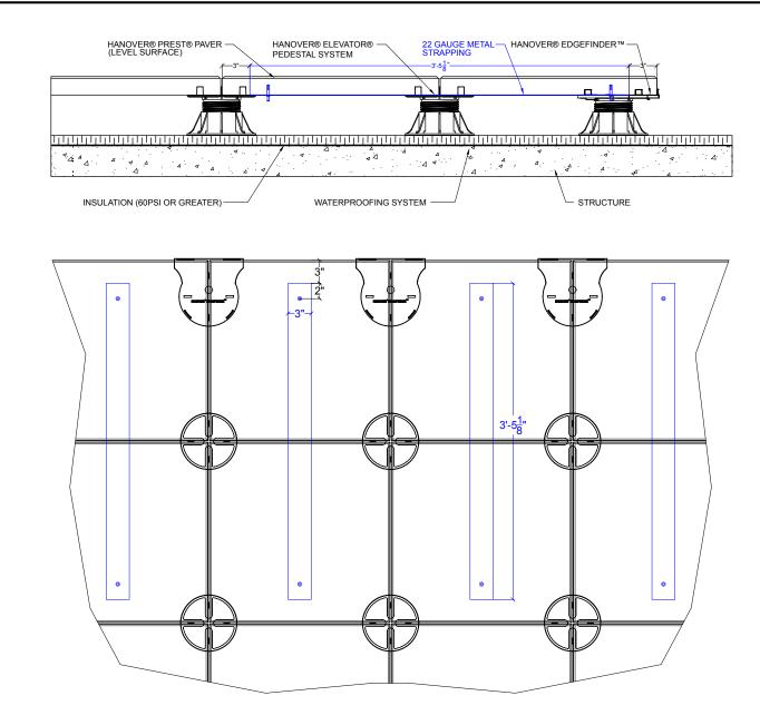
\* Hanover® requires the first two rows of pavers to be strapped together when using Hanover® EdgeFinder™. Hanover® recommends the use of a 3" wide, 22 gauge flat stainless steel strap at a length of 41 1/8". It is to be anchored to the underside of the pavers using a Zamac Nailin 1/4" x 1 1/4", all metal, provided by Powers Rawl part #2814. See drawing.
